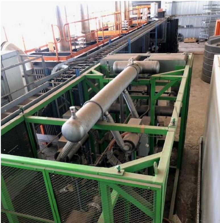
gTET ORC Generator in position. Pyrolysis equipment in the background.
