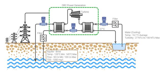
gTET has significant experience in binary cycle electricity generation gained from a variety of projects it has undertaken using its unique Organic Rankine Cycle (ORC) generators designed and manufactured at its headquarters in Victoria. The generation of power using gTET ORC generators is not limited to geothermal, many forms of waste heat can be used to generate electricity.
