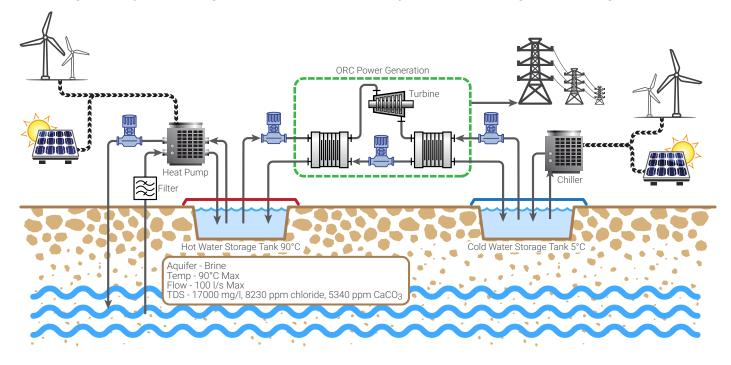
Image of a system using water as a thermal battery shown in underground storage tanks.
